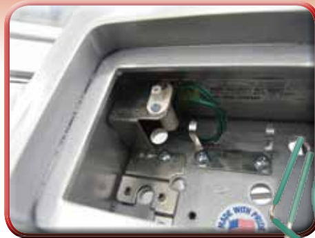
Closeup of a tamper switch for a recess mount Knox-Box®. Recess mounted Knox devices require only a door tamper switch. Wall mounted devices accommodate both door and rear tamper switches.
