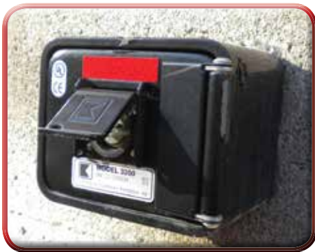
This KNOX-BOX® withstood significant physical attack by a sledgehammer. The last but most important security feature of a KNOX-BOX is PROPER INSTALLATION.
