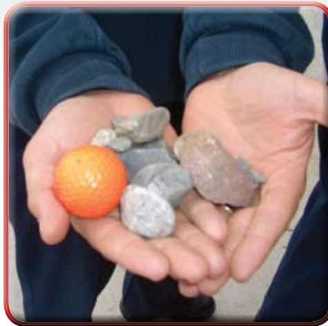
Debris removed from FDC connection
